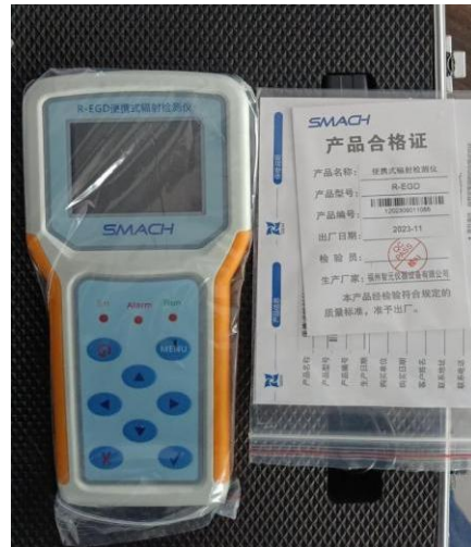
R-EDG型便携式辐射检测仪
